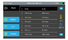
Select [Splice Option], choose the suitable splice option and press the Select button (the yellow font is the currently selected splice option)
